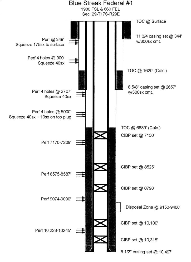
Drill out 4 squeeze jobs, drill out 3 CIBPs & squeeze 3 sets of perfs, then perforate & acidize Disposal Zone.
