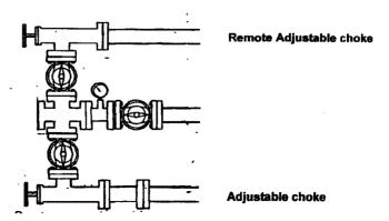
2" min 5000 psi Double valve manifold
