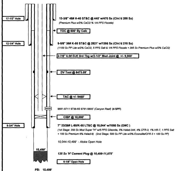
Drilled 6-1/8" Open Hole @ 10,044-11,075'. Set 135 Sx 'H' cement plug @ 10,499-11,075'. Ran tubing. Turned to production flowing Nov '97
