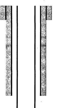
17-1/2" hole @ 694' 13-3/8" csg @ 694' w/715sx-TOC-Surf-Circ
