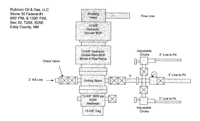
3000 psi Working Pressure BOPE Configuration And Choke Manifold
