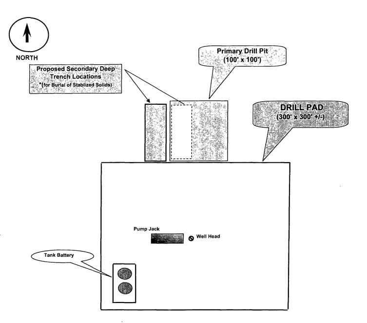
Note: Location of solids burial trench will be determined in the field based on site conditions, i.e. (terrain slope, vegetatation, etc.)
