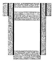
17-1/2" hole @ 400' 13-3/8" csg @ 400' w/585sx-TOC-Surf-Circ
