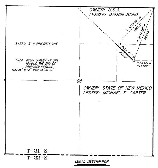
A STRIP OF LAND 30.0 FEET WIDE, LOCATED IN SECTION 32, TOWNSHIP 21 SOUTH, RANGE 28 EAST, N.M.P.M., EDDY COUNTY, NEW MEXICO AND BEING 15.0 FEET LEFT AND RIGHT OF THE FOLLOWING DESCRIBED CENTERLINE SURVEY.
