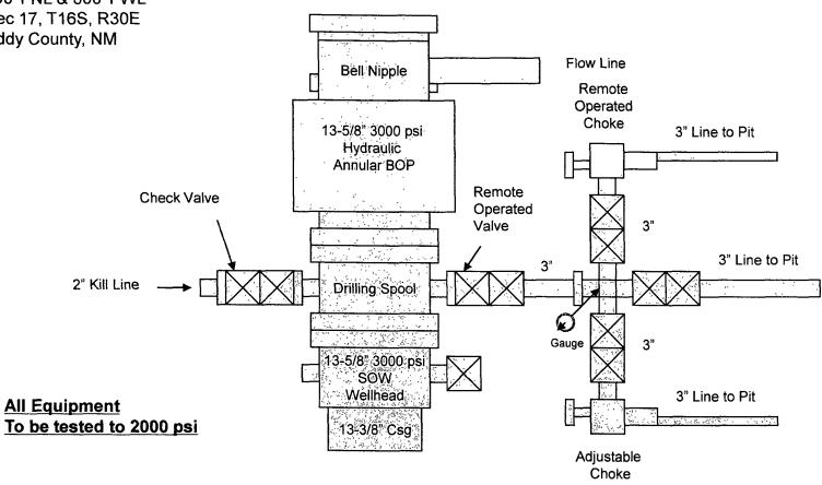
2000 psi Working Pressure BOPE Configuration And Choke Manifold
