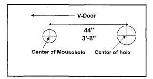
Notes for Rotating Mouse hole for a FlexRig3 & 25' Substructure:
