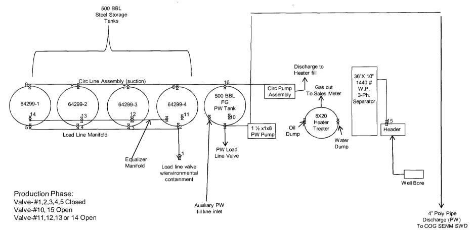
Sales Phase: Valve-#1 Open Valve-#2,3,4 or 5 Open Valve-#6,7,8,9 Closed Valve-#11,12,13,14 Closed
