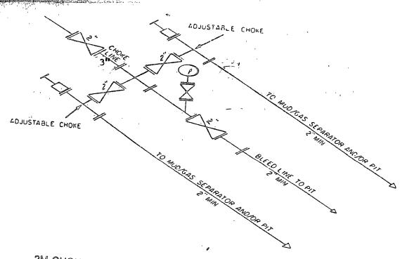
2M CHOKE MANIFOLD EQUIPMENT — CONFIGURATION OF . CHOKES
