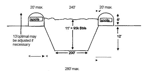
Spoil piles= 3 sides will normally be narrow and the fourth side will include the road and access to the sump. Bottom Slope- make sure the bottom always slopes to the sump. Top Edge= Make sure top levels are shot in to ensure adequate Free Board (2') Road & Ramps = Must be capable of handling 2 loaded water trucks.
