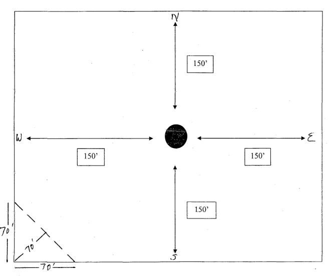
Portion of pad to be cut off to allow for diversion of drainage (SW corner of pad)
