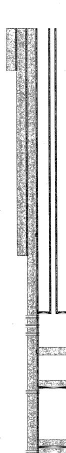
17-1/2" hole @ 810' 13-3/8" csg @ 810' w/ 1000sx-TOC-Surf-Circ
