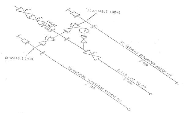
3M CHOKE MANIFOLD EQUIPMENT - CONFIGURATION OF CHOKES
