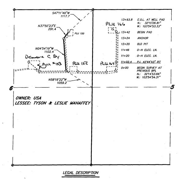
A STRIP OF LAND 30.0 FEET WIDE, LOCATED IN SECTION 6, TOWNSHIP 24 SOUTH, RANGE 30 EAST, N.M.P.M., EDDY COUNTY, NEW MEXICO AND BEING 15.0 FEET LEFT AND RIGHT OF THE ABOVE PLATTED CENTERLINE SURVEY.
