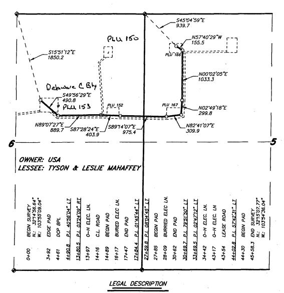
A STRIP OF LAND 30.0 FEET WIDE, LOCATED IN SECTIONS 5&6, TOWNSHIP 24 SOUTH, RANGE 30 EAST, N.M.P.M., EDDY COUNTY, NEW MEXICO AND BEING 15.0 FEET LEFT AND RIGHT OF THE ABOVE PLATTED CENTERLINE SURVEY.
