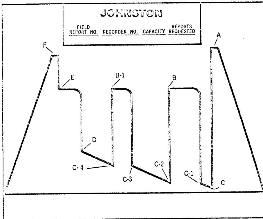
The following points are either fluctuating pressures or points indicating other packer settings, (testing different zones).
