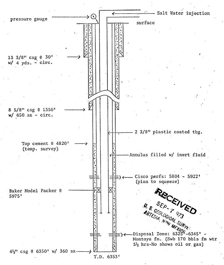
DIAGRAMATIC SKETCH of proposed installation of Water Injection Equipment for Read & Stevens Inc. No. 1 Federal "L" located 660' FNL & 1980' FEL, Section 21, T-6-S, R-27-E, Chaves County, New Mexico.
