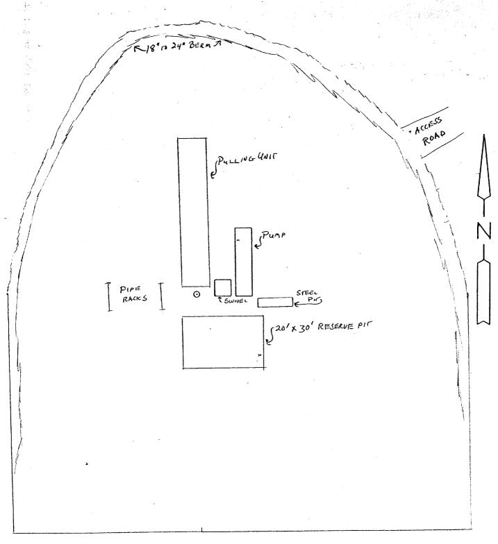
100' NORTH FROM CENTERHOLE 100' EAST FROM CENTERHOLE 90' South FROM CENTERHOLE 70' WEST FROM CENTERHOLE DRAWING NOT TO SCALE
