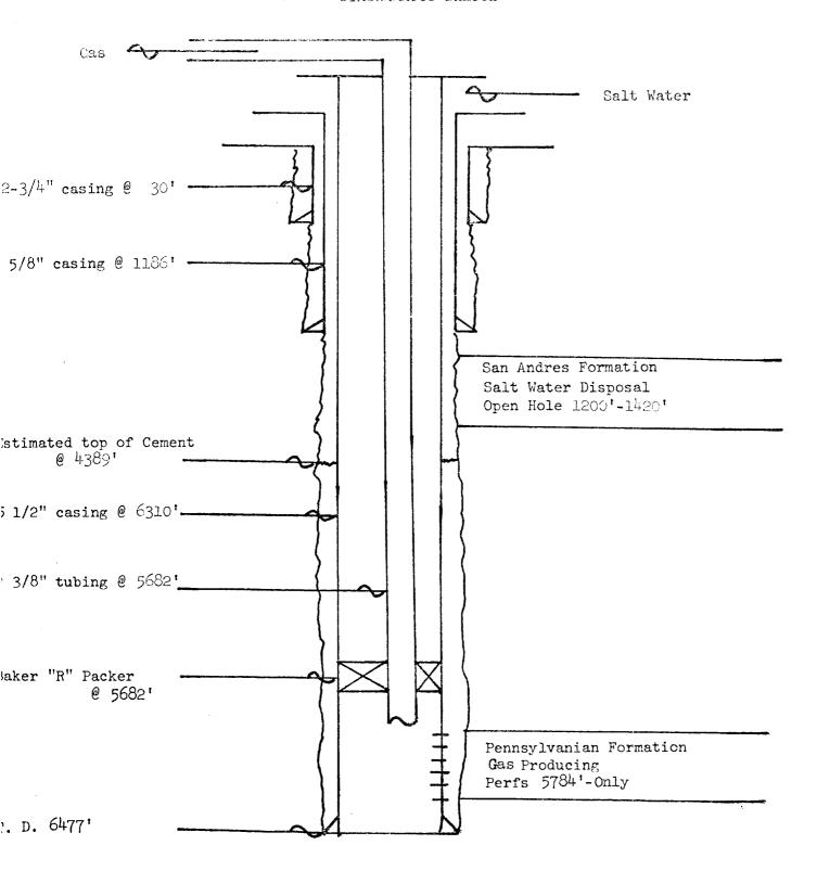
BLACKROCK OIL COMPANY Proposed Dual Completion Bates McIntyre Federal No. 1 Haystack Cisco Field Chaves County, New Mexico Unit H, Sec. 9, T-6-S, R-27-E
