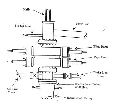
Typical 2,000 psi choke manifold assembly with at least these minimun features
