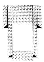
4" OD DRY HOLE MARKER 4' AGL CASING STUBS CUT OFF 3' BGL
