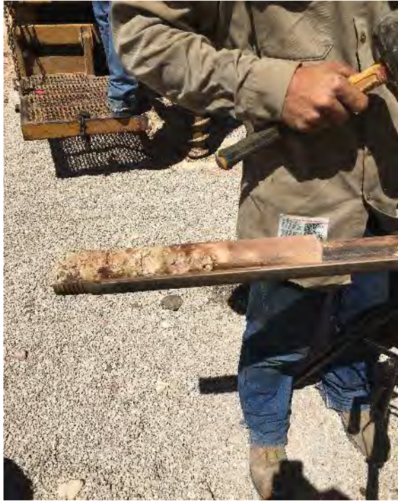
Photo 2: Interface of Dark Brown Clay and Caliche or Limestone rock encountered at 5 ft. bgs in V1.
