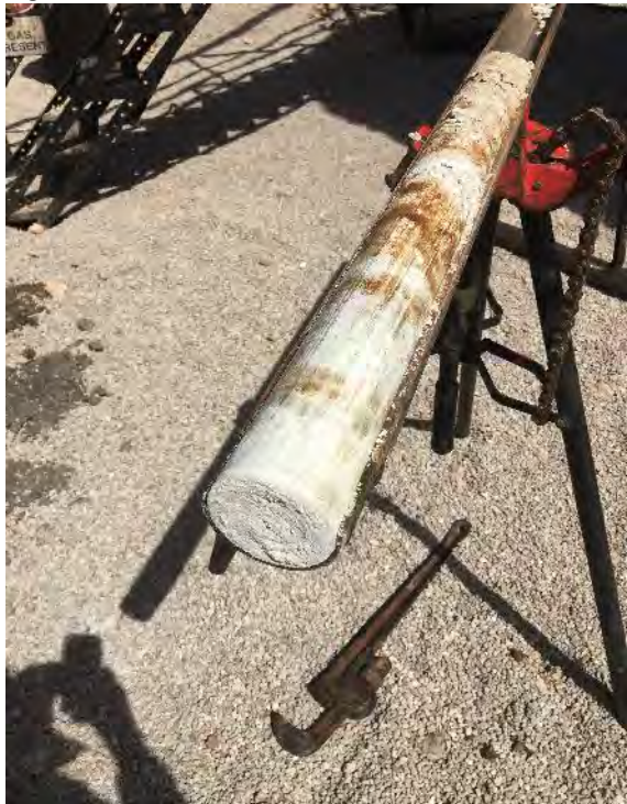
Photo 4: White limestone observed in the 15-20 foot interval of V1.
