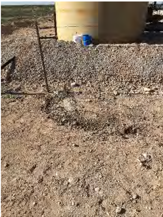
Photo 7: Closed soil boring location ES2.
