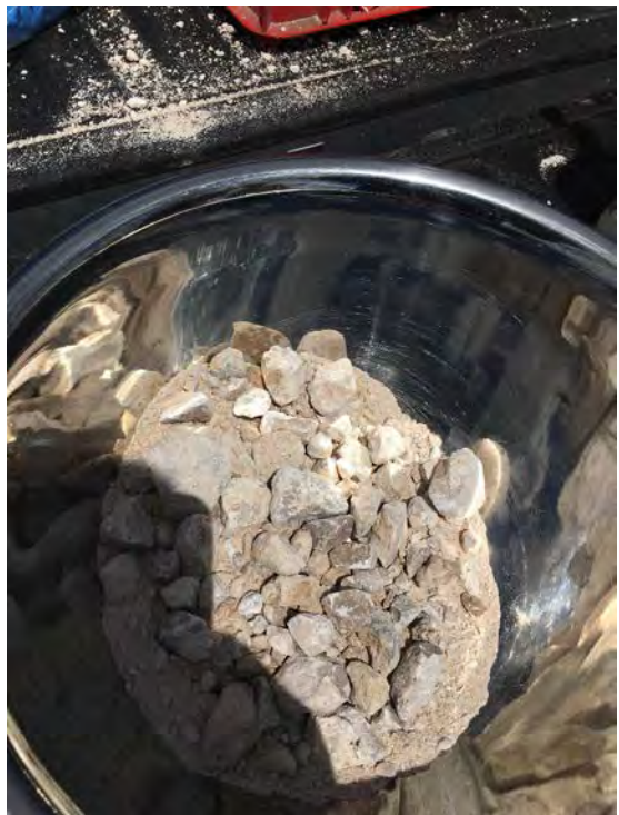
Photo 4: Slough materials retrieve in the 30 foot interval where hard rock was encountered.
