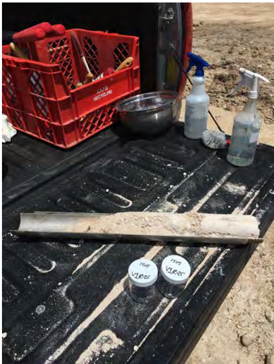
Photo 3: White limestone in the 25 foot interval of sample V1R-25.
