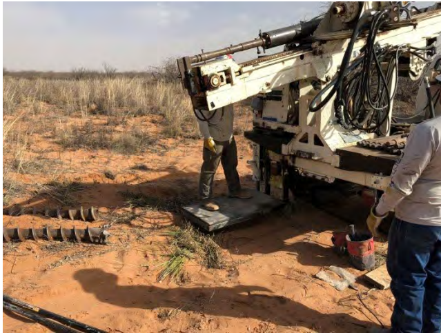
Photo 3: View of typical boring installed via geoprobe.
