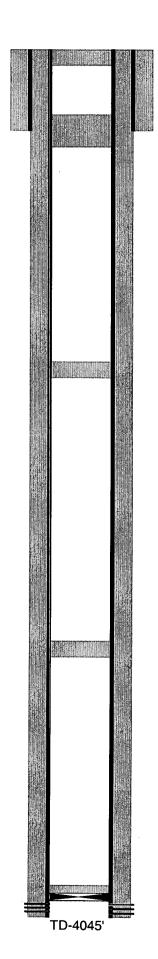
12-1/4" hole @ 385' 8-5/5" csg @ 385' w/250sx-TOC-Surf-Circ
