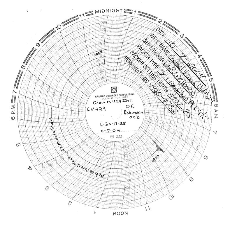
CHEVRON + TEXECT C.V.M. NO. 29 138-Jts 23/8-J-SS-NOULING T.B. q. 4370.70 Ft. 2-Subs 23/8× 6:00 Ft. 423/2×10:00 Ft. Set @ 4402. 85 Parts 4460-4752 CS9, 4/2 10:57
