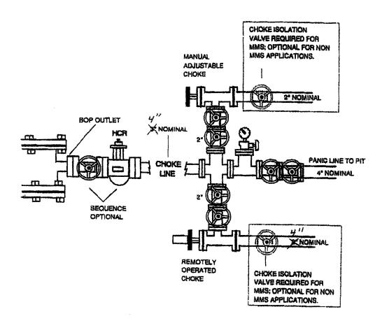
Exhibit E Continued **Blowout Preventor Choke Manifold** Pipeline Deep 7 Federal Com No. 2 Gruy Petroleum Management Co. Unit P-Section 7-T19S-R34E 1210' FSL & 1215' FEL Lea County, NM
