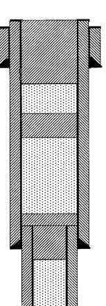
4. PUH to 375' & spot 100 sx Class "C" cmt from 375' to surf (Casing leak, Shoe, & Water Board)
