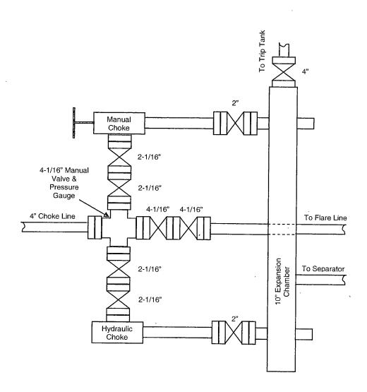
Profile View of Piping from Choke Manifold to the Mud Gas Separator
