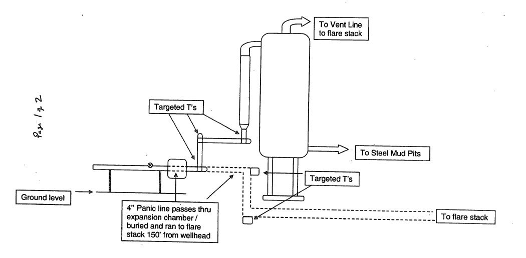
Aerial View of the Piping from the Choke Manifold to the Mud Gas Separator
