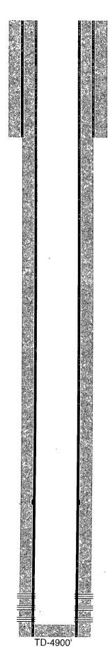
12-1/4" hole @ 820' 9-5/8" csg @ 820' w/ 450sx-TOC-Surf-Circ
