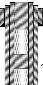
4. PUH to 308' & spot 55 sx Class "C" cmt from 308' to surf. (Shoe & Water Board)
