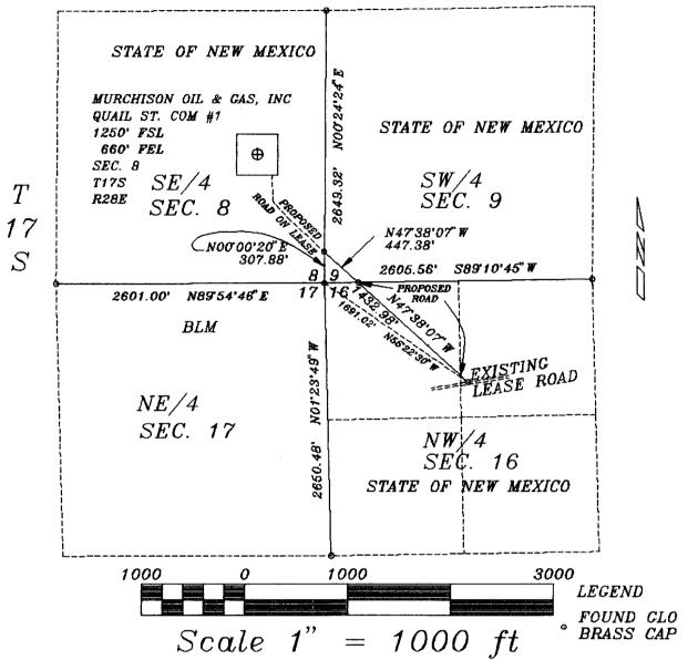
BASIS OF BEARING: NEW MEXICO STATE PLANE COORDINATE SYSTEM (EAST ZONE NAD 1983)
