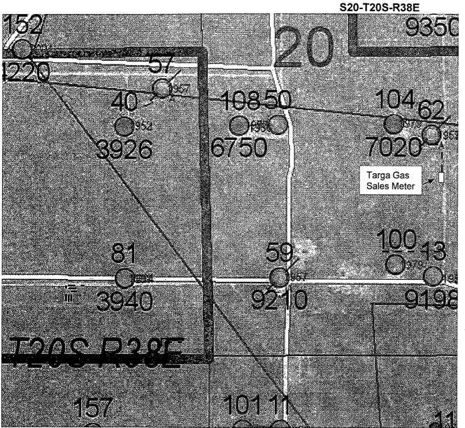
Gas line installation will be 3", SDR 7, buried, black polyethylene pipe. Pipe to be buried 3' deep with tracer wire.
