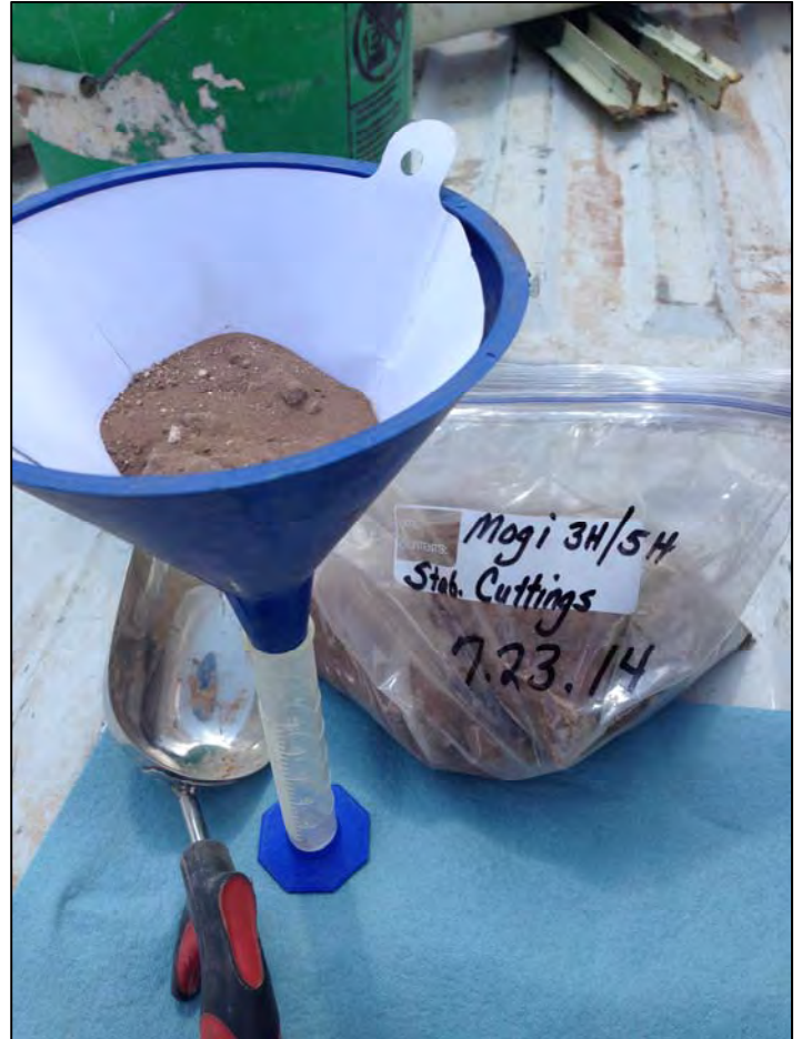
Paint filter test on stabilized cuttings 7/23/2014
