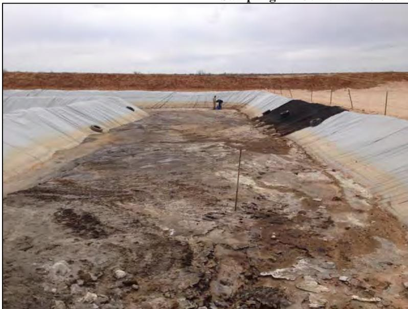
stabilized cuttings” by mathematically combining 1 part pit contents and 3 parts clean soil (mixing dirt). The weighted pit composite calculation consists of 25% solids from the inner cell of the drilling pit and 75% of the solids from the outer cell (1:3 ratio), representative of the volume of cuttings in each cell.
