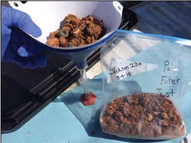
Paint filter test on stabilized cuttings
