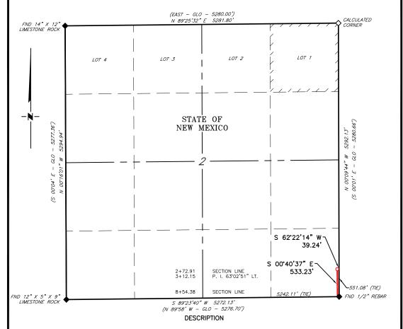
A strip of land 20 feet wide, being 572.47 feet or 34.695 rods in length, lying in Section 2, Township 10 South, Range 36 East, N. M. P. M., Lea County, New Mexico, being 10 feet left and 10 feet right of the following described survey of a centerline across State of New Mexico land:
