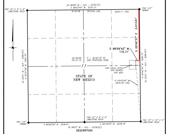
A strip of land 20 feet wide, being 2,586.32 feet or 156.746 rods in length, lying in Section 11, Township 10 South, Range 36 East, N. M. P. M., Lea County, New Mexico, being 10 feet left and 10 feet right of the following described survey of a centerline across State of New Mexico land:
