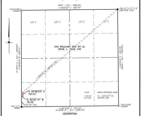
A strip of land 20 feet wide, being 272.91 feet or 16.540 rods in length, lying in Section 1, Township 10 South, Range 36 East, N. M. P. M., Lea County, New Mexico, being 10 feet left and 10 feet right of the following described survey of a centerline across the lands of Joe Williams EDD ET. AL. according to a deed filed for record in Book 1, Page 330, of the deed records of Lea County, New Mexico:
