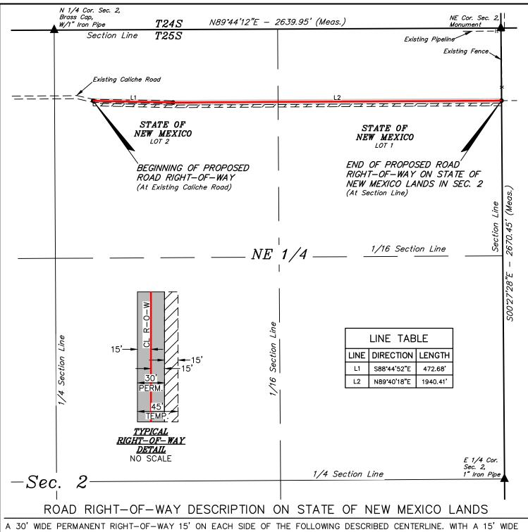
A 30' WIDE PERMANENT RIGHT-OF-WAY 15' ON EACH SIDE OF THE FOLLOWING DESCRIBED CENTERLINE. WITH A 15' WIDE TEMPORARY RIGHT-OF-WAY ON THE RIGHT SIDE OF SAID PERMANENT RIGHT-OF-WAY.
