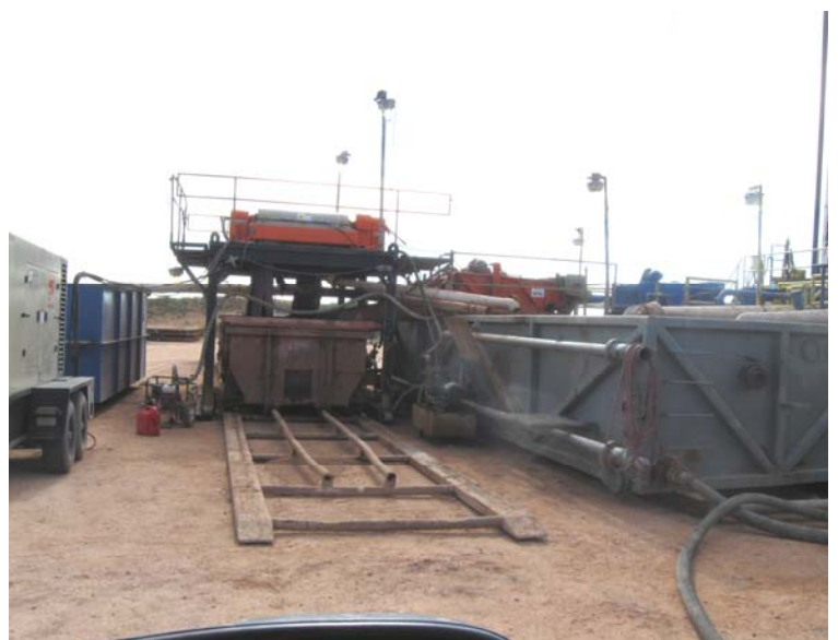
Above: Centrifugal Closed Loop System
