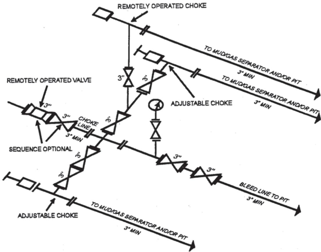
10M AND 15M CHOKE MANIFOLD EQUIPMENT - CONFIGURATION OF CHOKES MAY VARY
