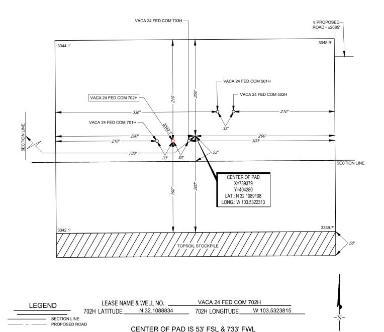
ALL BEARINGS, DISTANCES, AND COORDINATE VALUES CONTAINED HEREON ARE GRID BASED UPON THE NEW MEXICO COORDINATE SYSTEM OF 1983. EAST ZONE, U.S. SURVEY FEET.
