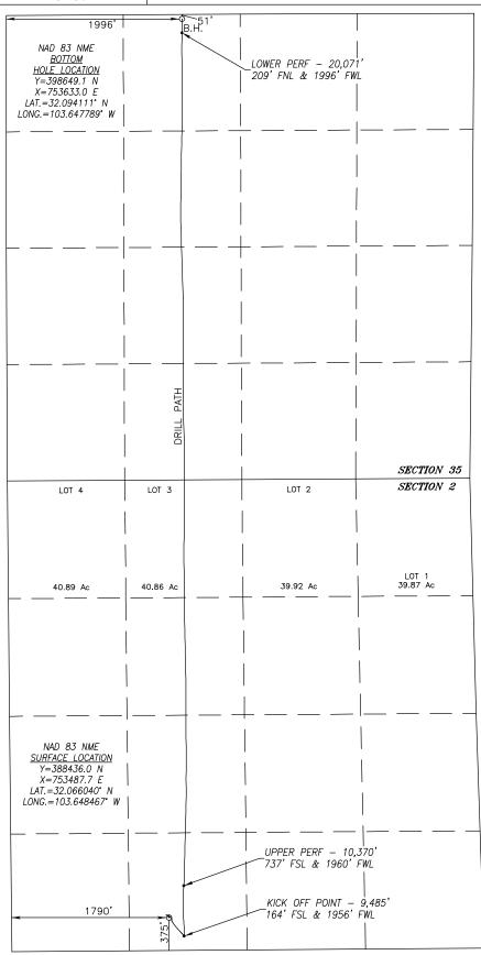
SURFACE INFO AND BOREPATH SHOWN HEREON IS BASED ON DIRECTIONAL SURVEY REPORT PROVIDED BY COG OPERATING, LLC FOR THE HARRIER FEDERAL COM #302H SUPPLIED TO HARCROW SURVEYING, LLC ON JUNE 2, 2020
