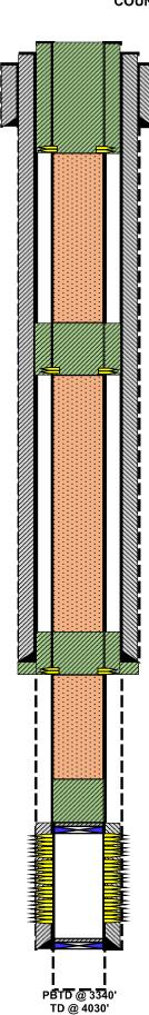
4. PUH & perf @ 300' & sqz/CIRC 90 sx Class "C" cmt from 300' to surf. (Water Board, Surf Shoe, & Surf Plug)
