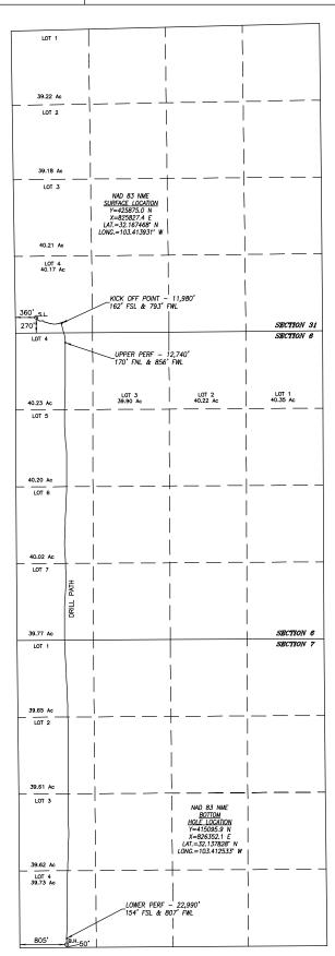
SURFACE INFO AND BOREPATH SHOWN HEREON IS BASED ON DIRECTIONAL SURVEY REPORT PROVIDED BY COG OPERATING, LLC FOR THE STOVE PIPE FEDERAL COM \$706H SUPPLIED TO HARCROW SURVEYING, LLC ON SEPTEMBER 3, 2020
