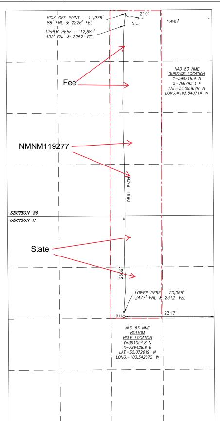
SURFACE INFO AND BOREPATH SHOWN HEREON IS BASED ON DIRECTIONAL SURVEY REPORT PROVIDED BY COG OPERATING, LLC FOR THE VALOR FEDERAL COM 704H SUPPLIED TO HARCROW SURVEYING, LLC ON JANUARY 27,
