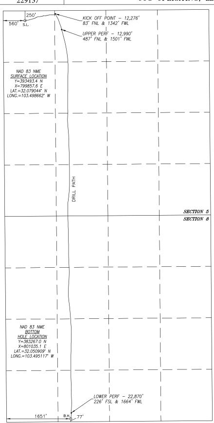
SURFACE INFO AND BOREPATH SHOWN HEREON IS BASED ON DIRECTIONAL SURVEY REPORT PROVIDED BY COG OPERATING, LLC FOR THE GUNNER B FEDERAL COM #804H SUPPLIED TO HARCROW SURVEYING, LLC ON JANUARY 4,
