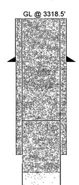
Pumped 75 sx into surface-prod csg annulus; circ to surf Cmt level after 6 hrs: full
