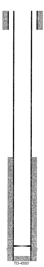
17" hole @ 329' 13-3/8" csg @ 329' w/ 325sx-TOC-Surf-Circ
